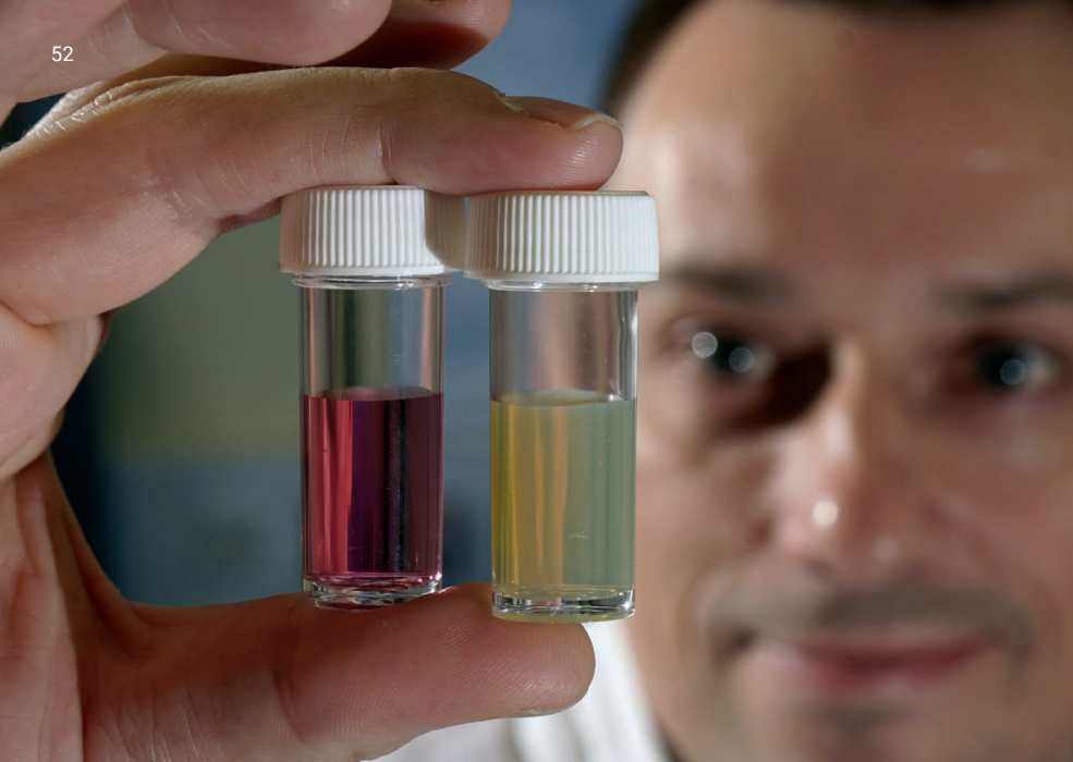
As part of a new project, Dr Thomas Schneider is synthesizing and characterizing nanoparticles—here he presents solutions with nanospheres made of gold (left) and silver.
